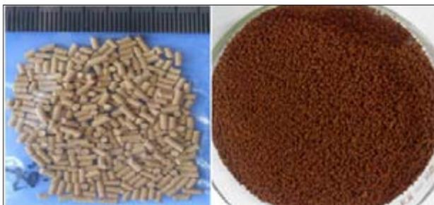
Particulate Fe-Al-Ce (left) and Mg-Fe-Ce (right) fluoride removal adsorbents
