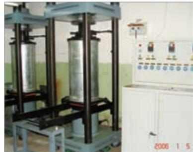
Creep testing system for fully-graded concrete
