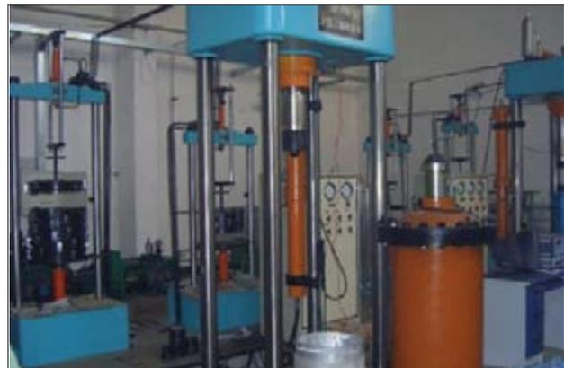
Independently designed and developed SR-4 mile-controlled high-pressure triaxial rheometer
