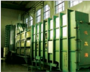
Vacuum tank (vacuum percentage 98.7%; flow discharge 1.0 m<sup>3</sup>/s)
