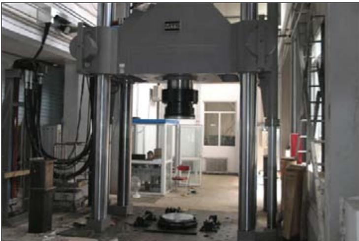
*Large-scale Testing Machine for Dynamic Performance of Full-grade Concrete*
