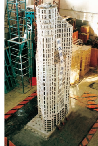
Dynamic experiment of Nanjing World Trade and Exhibition Center on Shaking Table
