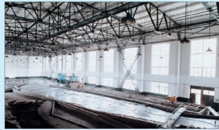
Movable bed model test on the confluent region of Weihe and Luohe Rivers in the middle reach of Yellow River
