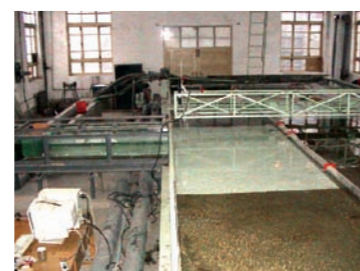
Sedimentation and pollution control test for water intakes of thermal/nuclear power stations
