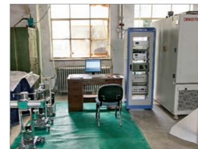
Frost-break testing of asphalt concrete
