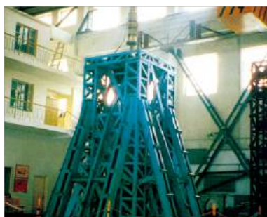
Tri-axial earthquake simulating shaking table with 6 degrees of freedom
