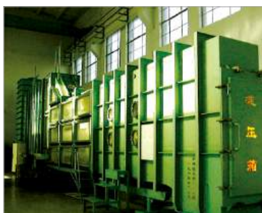
Vacuum tank (vacuum percentage 98.7%; flow discharge 1.0 m 3 /s)
