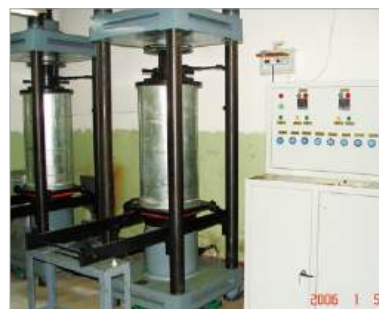
Creep testing system for fully-graded concrete
